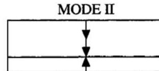
Mode II - Crack propagates up to reinforcement, then starts again from top of sample and propagates downward
