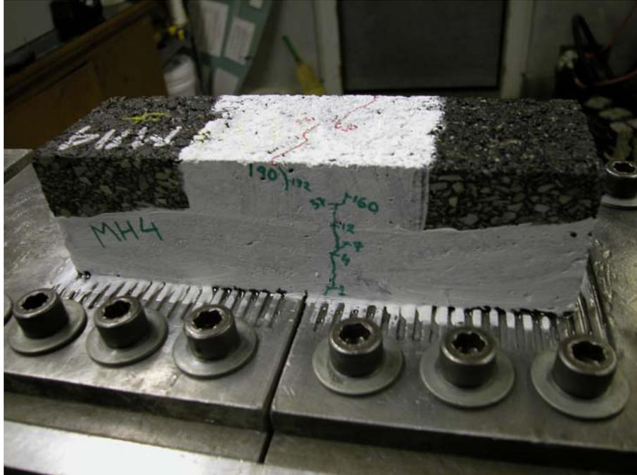
Specimens containing a complete FiberMat system (bond coat - fiber - bond coat - stone) mostly had cracks that propagated by means of horizontal cracks along the interlayer – see photo below. Before that, they survived much longer than the control specimens.
