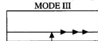
Mode III - Crack propagates to bottom of reinforcement and then is redirected horizontally
